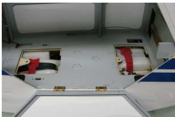
View of battery compartment under floor
