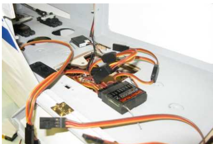
View of radio installation
